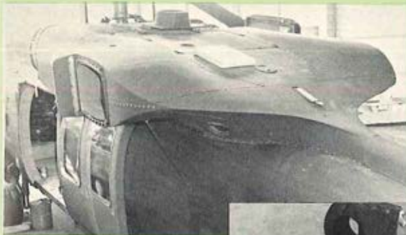
LEFT: The mounting of an IR suppressor kit increases survivability against heat-seeking missiles by reducing the IR signature and the line-of-sight view of hot metal engine parts.
