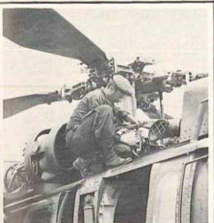
Non-skid walkways are provided on the forward crown area to facilitate maintenance for the hydraulic flight control, electrical, and heating systems. Hand-holds and steps are also provided to climb to the top of the BLACK HAWK safely.
