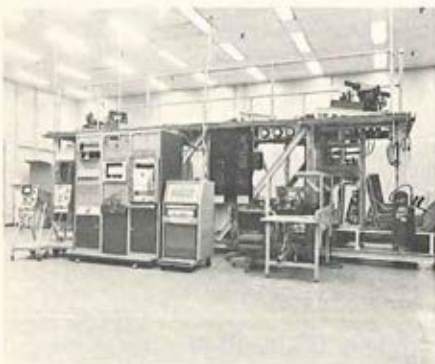
PHOTO ABOVE: The "Iron Bird" laboratory mockup that checks out the essential flight control hardware. BELOW: The CH-47D aft transmission that completed qualification testing.
