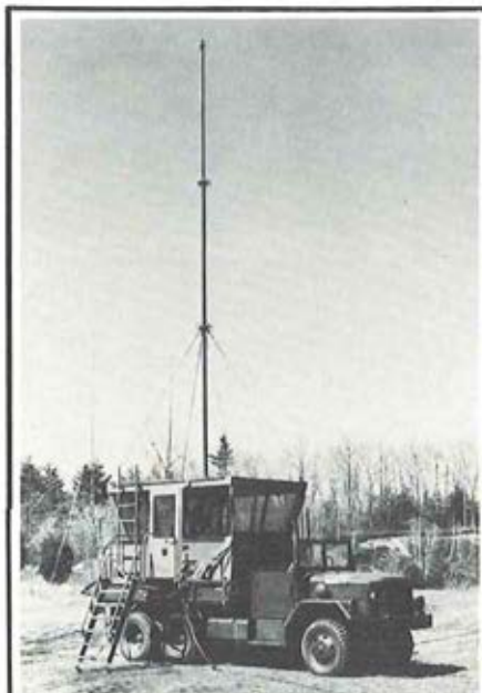
FIGURE 1—THREE-MAN AIR TRAFFIC CONTROL CENTRAL, AN/TSW-7A
