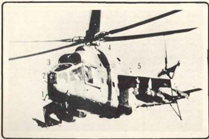
Left: An Mi-24 helicopter gunship. Mission: Fire support during assault landings. 1] Pitot Head 2] 12.7 mm machine gun. 3] Bullet-proof shield. 4; Engine exhaust 5] Laser rangefinder on gun camera mount. 6] Pods holding 32.57-mm unguided rockets, and 7] Rails for 'Swatter' semi-automatic ATGW. — Encycl. of Land Warfare.
