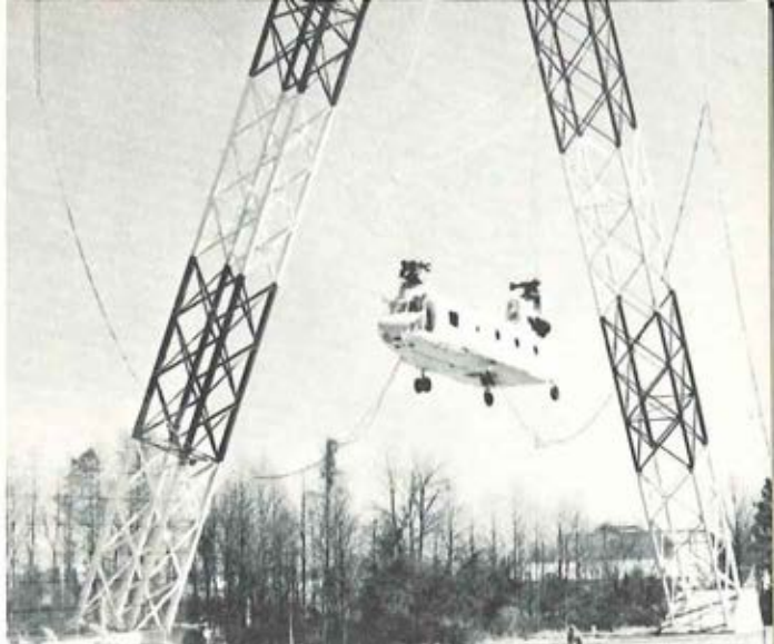
Figure 4 Army-NASA Drop Crash Testing at Langley Test facility. The CH-47C is shown prior to impact.
