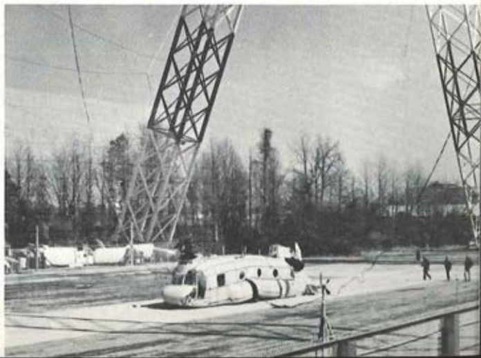
Figure 5 The CH-47C undergoing drop testing is shown after impact at the Langley drop test facility.
