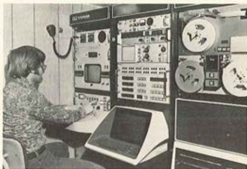
Pictured at the PATS console is the single operator needed to measure range, azimuth, and elevation of airborne test vehicles with cost-efficient accuracy.
