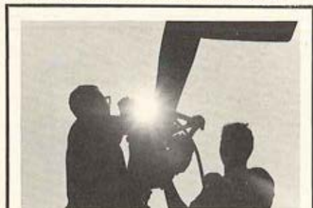
FINAL PREPARATIONS - SP4 Rick Smart (left) and Dave Napheney, Co C, 159th Avn Bn of the 101st, take off a tail rotor of a Chinook during port operations at Norfolk Naval Base, Va. The 'copter was one of 318 being readied for sea-lift to Europe for REFORGER 76.
