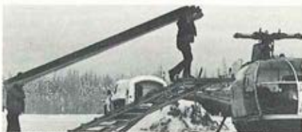
Mechanics re-attach Alouette blades each a.m.
