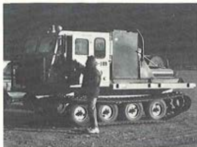
□ The fire truck at the Camp Dietrich airstrip is a tracked Canadian-made vehicle. Such equipment is necessary since there is virtually no road access to the area in which the fire is located once one goes beyond the immediate camp ground itself. □
