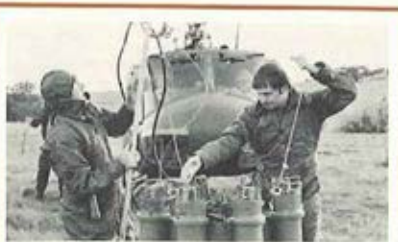
LOAD 'EM UP! — Art White, left, and Don R. Brandt, Picatinny Arsenal Engineers, prepare a 155mm flare dispenser for loading during a MASSTER battle-field illumination test. The dispenser is one of a number of night vision devices being tested to evaluate the relationship between artificial illumination and the night vision devices. [USA photo]
