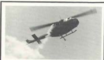
TEST RUN—Using a smoke device to show wind patterns, an Army Huey also dispenses a load of chaff — small metallic and fiberglass strips that are used to distort and confuse enemy radar. The chaff is also being dropped to determine its effects on aircraft engines. Testing is being conducted at Ft. Hood under MASSTER. [USA photo]
