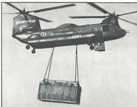
"Fly-by-wire" flight tests—HLH test bed
