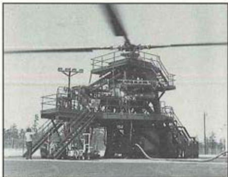
Dynamic system test rig
