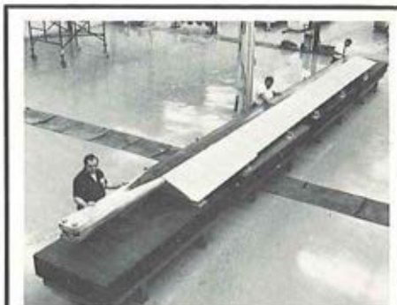
THE BIGGEST! —The Boeing Vertol Company achieved a milestone last week with the fabrication of the free world's largest helicopter rotor blade. One of eight on the Army's XCH-62 Heavy Lift Helicopter, the big blade is 41.5 feet long and will weigh 750 pounds in its flight configuration.
