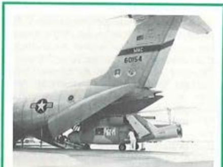
TRANSPORTABILITY — An airlift capability characterizes tomorrow's UTTAS. Here two Boeing UTTAS helicopters with rotor blades and tail booms folded are airlifted easily in a C-141.
