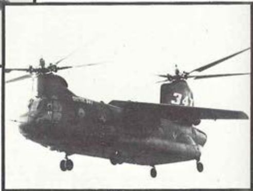
PHILADELPHIA, PA. — The first flight of the world's largest tandem helicopter with a controllable tilt-wing-Boeing's 347 — took place on January 26 at Boeing's Flight Test facility in Ridley Township. The winged 347 with its 340 sq. ft. wing, is designed to demonstrate improved maneuverability at design cruise speeds (170 knots) and mission weights (45,000 lbs). The Army-supplied CH-47A Chinook's length was extended 110 inches, as one of several modifications.
