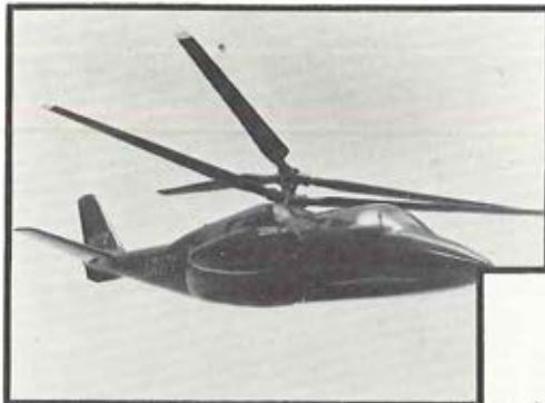
PHILADELPHIA, PA. — The first flight of the world's largest tandem helicopter with a controllable tilt-wing-Boeing's 347 — took place on January 26 at Boeing's Flight Test facility in Ridley Township. The winged 347 with its 340 sq. ft. wing, is designed to demonstrate improved maneuverability at design cruise speeds (170 knots) and mission weights (45,000 lbs). The Army-supplied CH-47A Chinook's length was extended 110 inches, as one of several modifications.
