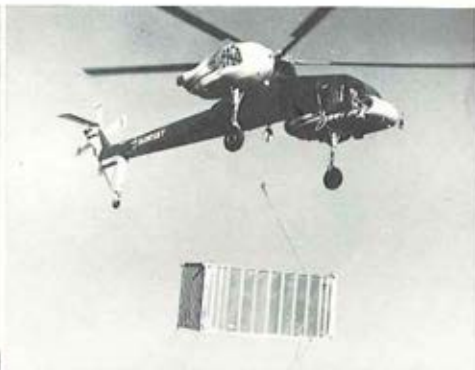
2. 1959. We built the world's first heavy-lift crane-type helicopter, the 5-ton payload S-60.
