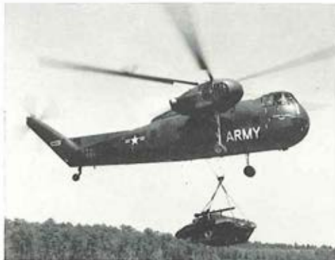
1. 1953. We built the first production heavy-lift helicopter, the S-56 (CH-37). It had a payload of 3 tons—more than any other copter then flying.
