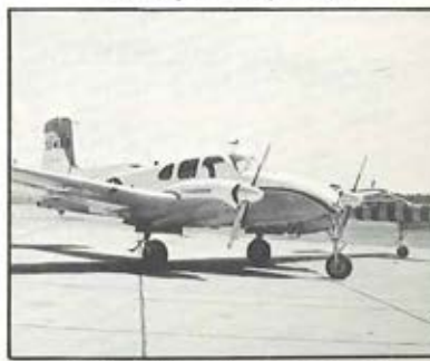
L-23 with fuel tank outriggers
