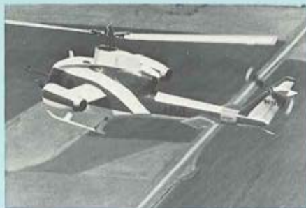
FORT WORTH — The Bell Helicopter Company announced on April 28 that its compound search helicopter (above) had set a record speed of 316 MPH (274.5 knots) in level flight. The modified YH-40 has a Lycoming T53-L13 as its primary engine and two Pratt & Whitney JT12-A3's, with 3,300 pounds static thrust each, on its wing tips. (Bell photo)
