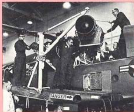
VAN NUYS — U.S. Army students — all veteran helicopter maintenance men — remove a gas turbine engine from a new AH-56A Cheyenne during the first instruction course for mechanics and technicians who'll support the advanced gunship. The new school has been established at the Van Nuys plant of the Lockheed-California Company, developer of the Cheyenne. At lower left, Lockheed instructor Charles LaMarr gives students a few pointers in procedure. Trained personnel are expected to remove a Cheyenne engine in approximately thirty minutes. (Lockheed)
