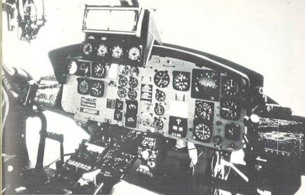
ABOVE: Light Low Level TV (interior view) as shown installed in a UH-1C Iroquois. Reading scopes are shown at the right and left of the instrument panel.
