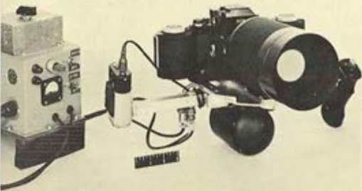
ABOVE: Airborne long focal length camera system (Experimental). Nikon camera with 500mm lens, Kenyon gyro. Shows camera with power supply.
