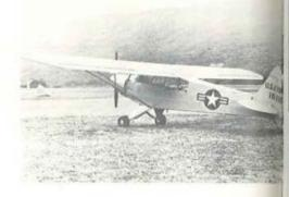
Army procured 150 A models and 69 B models. This metal-frame fabric-covered airplane was used mainly as a trainer. The B model saw extensive use in the Far East. The L-18C, purchased for MDAP, was the same as the L-21 except that it had a 90 hp. Continental engine.
