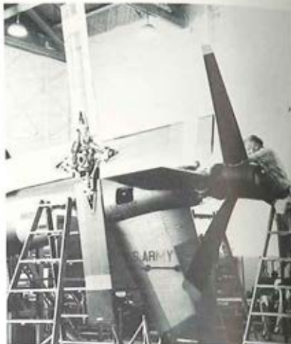
VAN NUYS — The free world's only helicopter-type aircraft with both a tail-mounted pusher propeller and rotor, this U.S. Army AH-56A Cheyenne nears completion in final assembly at Lockheed-California Company's Van Nuys plant. Other Cheyenne aircraft are now undergoing flight testing. The 250-mph AH-56A will "ride shotgun" for troop-carrying helicopters and provide direct fire support in the combat landing zones.
