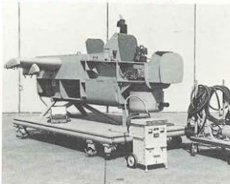
Weapons maintenance trainer and power supply cart
