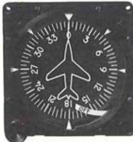
New ARC G-112A electric directional gyro gives you easy to read vertical card presentation and its 12"/hour drift rate exceeds TSO specifications. It only weighs in at 3 lbs. and you can mount it in panels inclined up to 10° without affecting specs.
