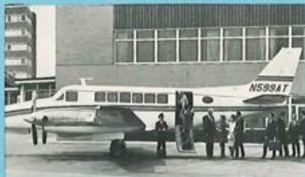
The largest airplane yet to be marketed by Beech, the 17-place turbine-powered Beechcraft 99 will enter production in Spring, 1968, for scheduled airline and air taxi markets. Powered by twin PT6A-20 turbines, the 99 cruises at 250 mph and has a maximum takeoff weight of 10,200 pounds.
