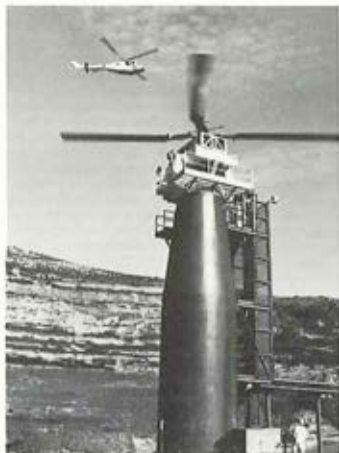
SAUGUS, CALIF. — The world's most powerful whirl test tower, Lockheed's 55-foot facility is capable of testing rotor blades up to 110 feet in diameter. A set of blades for the Army AH-56A helicopter is shown under test.
