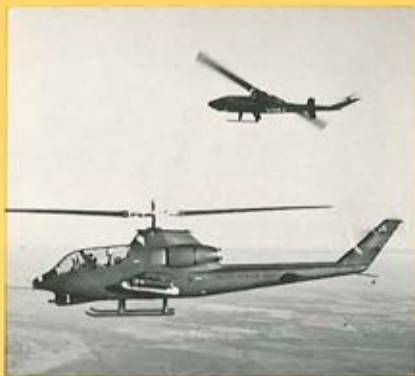
FT. HOOD — Now undergoing two-phase airworthiness qualification testing, two AH-1G HueyCobras prepare to dive during first phase jettison tests of rocket and machine gun pods carried under the stub wings. Some 300 pods of various configurations are being dropped over a five-week period to aid in assuring safe separation characteristics when a pilot jettisons pods in an emergency. Armament firing testing will constitute the second phase with Bell Company pilots handling the test aircraft throughout both phases. The tests are being conducted by Bell under contract to the Army Aviation Materiel Command.
