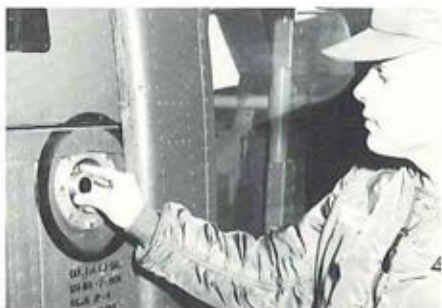
Automatic Shut-Off Nipple completely inserted in Adapter mouth
