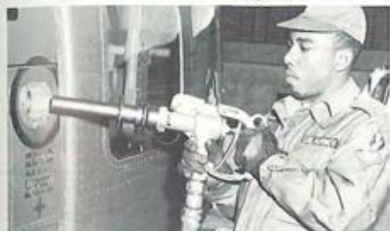
Automatic Shut-Off Nozzle attached to conventional refueling nipple
