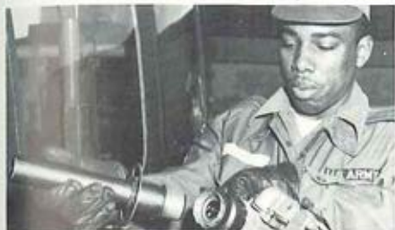
Automatic Shut-Off Nozzle being attached to conventional refueling nipple
