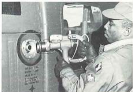
Automatic Shut-Off Nozzle being inserted for automatic shut off refueling operation
