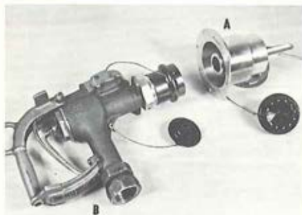
The complete automatic shut-off closed circuit refueling system is shown in the photo above. The aircraft adapter (A at top right) and the nozzle assembly (B). Individual dust caps are attached by cables. (USA photo)
