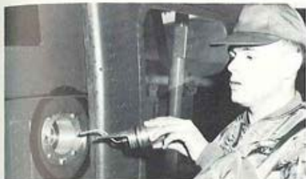
Automatic Shut-Off Nipple being removed to refuel conventionally
