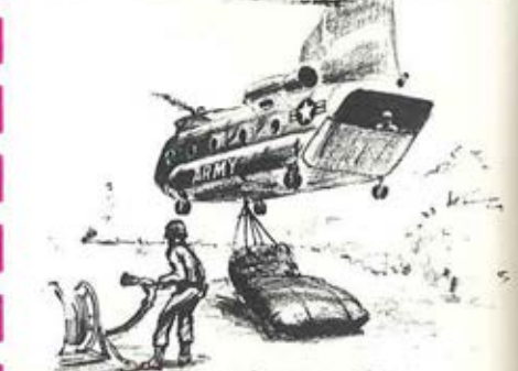
Chinook Brings 2,000 Gal. Air-Log Tank to Air-Log R.A.F.T.*
