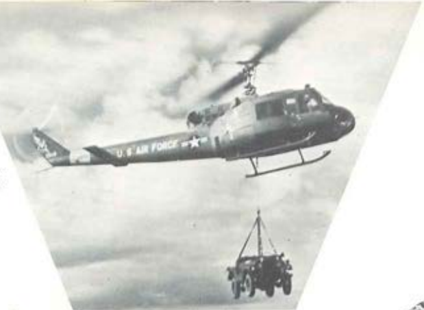
USAF Bell UH-1F utility helicopter powered by single G-E T58
