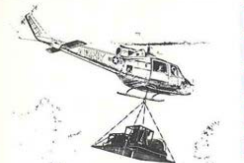
Air-Log Remote Area Fueling Terminal Delivered Forward by Huey
