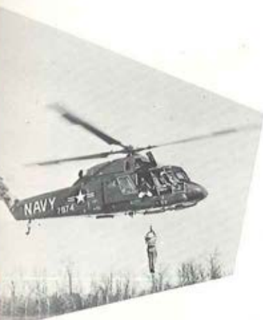
USN Kaman UH-2 utility helicopter powered by single G-E T58
