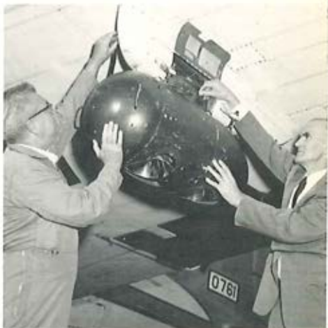
Units of the modified electronic flash system tested by the Army Electronic Command, Ft. Monmouth, N.J., to obtain night-time aerial color photos are examined by Francis Frame, left, assistant to electronic engineer, and Alvin F. Applegate. Tests proved the flash system to be effective up to 1,000 feet.
