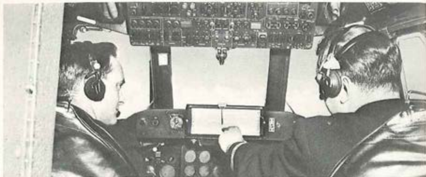
The Decca Flight Log indicator continuously presents current position and past track of the aircraft . . . the ultimate in pictorial presentation.
