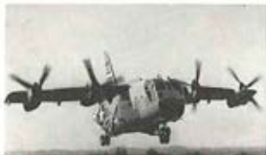
TILT-WING V/STOL TRANSPORT XC-142A has been developed by the three-company team of Ling-Temco-Vought, Hiller and Ryan for Army, Navy and Air Force. It will be capable of transporting troops and equipment into unprepared areas under all weather conditions.
