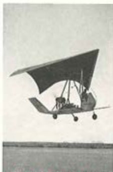
FLEX WING STOL "FLEEP" , popular name of the easy-to-fly XV-8A, is under study by Army's Transportation Research Command as an aerial "truck," capable of operating in areas where terrain conditions are rugged.
