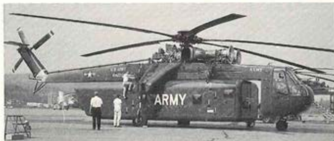
Sikorsky-built U. S. Army YCH-54As can lift large detachable troop vans. Other vans can serve as repair shops, command posts, hospital units.
