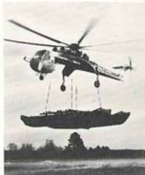
The Army's 11th Air Assault Division is using YCH-54As to develop a concept of heavy lift. Above, the 11th Air Assault tests lifting a class 60 pontoon bridge.
