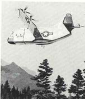
TILT-WING V/STOL TRANSPORT XC-142A is being built by Ryan (jointly with Vought and Hiller) for Army, Navy and Air Force. It will be capable of transporting troops and equipment into unprepared areas under all weather conditions.
