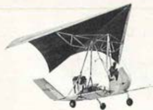
FLEX WING STOL "FLEEP," popular name of the easy-to-fly XV-8A, is under study by Army's Transportation Research Command as an aerial "truck," capable of operating out of rugged areas.
