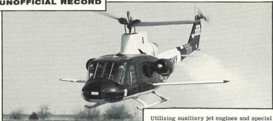
Utilizing auxiliary jet engines and special rotor blade tips, a modified YUH-1B compound helicopter flew 236 mph on Oct. 15 near Bell's Ft. Worth plant, unofficially breaking the Russian-held world speed record of 221 mph set in 1961. (Bell photo)
