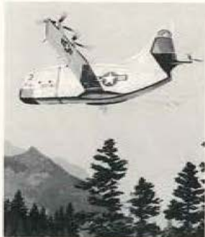
TILT-WING V/STOL TRANSPORT XC-142A is being built by Ryan (jointly with Vought and Hillier) for Army, Navy and Air Force. It will be capable of transporting troops and equipment into unprepared areas under all weather conditions.
