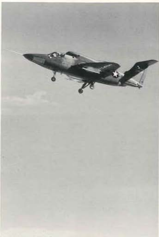
NEWEST RYAN V/STOL is Army XV-5A, lift-fan research aircraft built under contract to General Electric. Designed to take off vertically on no more power or fuel than is needed for high speed cruise, the XV-5A is now in flight test.
