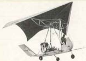
FLEX WING STOL "FLEXP," popular name of the easy-to-fly XV-8A, is under study by Army's Transportation Research Command as an aerial "truck," capable of operating out of rugged areas.
