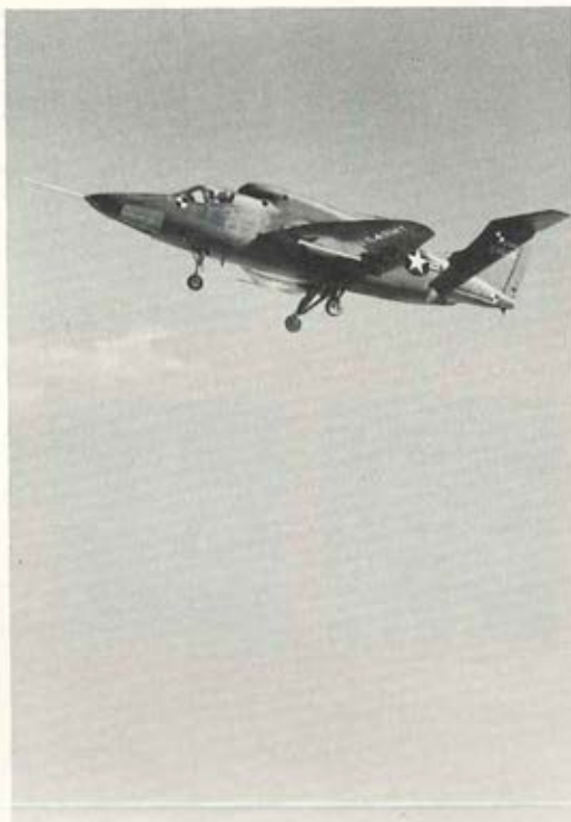
NEWEST RYAN V/STOL is Army XV-5A, lift-fan research aircraft built under contract to General Electric. Designed to take off vertically on no more power or fuel than is needed for high speed cruise, the XV-5A is now in flight test.
