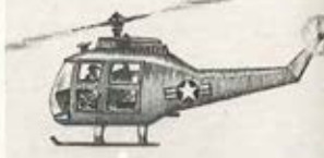
Turboshaft version of the T63 which is powering Light Observation Helicopters.
