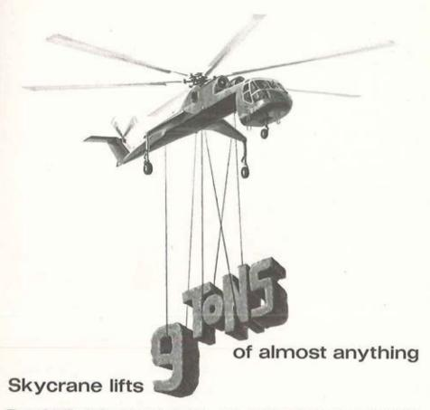
The new S-64 Sikorsky Skycrane, now in test, is a heavy-duty helicopter capable of lifting an astonishing variety of 9-ton loads of almost any shape.
