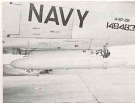
CLOSE-UP PHOTO OF DRAG CHUTE INSTALLATION ON THE TEST A4D JET AIRCRAFT.
