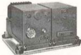
R-34A RECEIVER, powered by DV-10A Dynaverter, shown with B-13A-1 CONVERTER on E-14 RACK and M-10 MOUNTING
