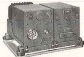
R-34A RECEIVER, powered by DV-10A Dynawerter, shown with B-13A-1 CONVERTER on E-14 RACK and M-10 MOUNTING
