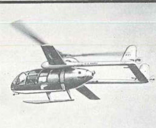
McDonnell XV-1 (Army). The world's first successful convertiplane. This research vehicle was an unloaded-rotor, compound helicopter combining hovering capability with a speed of 200 mph. The rotor was powered by McDonnell-designed blade-tip-mounted pressure jets.
