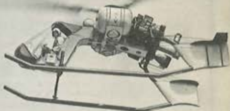
McDonnell Model 120. A "flying crane" of diminutive size but unusual lift capabilities. Powered with McDonnell rotor-tip-mounted pressure-jets, it can carry a useful load exceeding its empty weight. Military evaluation has shown outstanding hover and dynamic longitudinal stability for this experimental craft.
