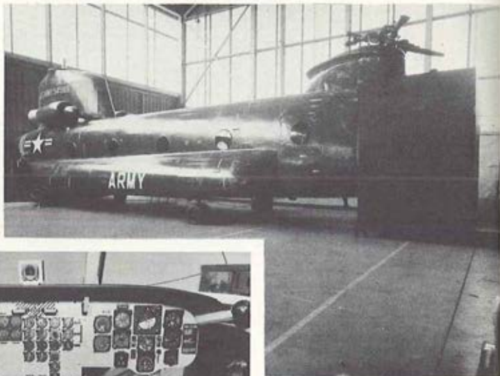
Chinook Mockup With Light-tight enclosure for nose section
