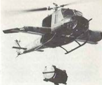
Demonstrating its ability to carry more than 3,000 lbs of parts to another ship hypothetically damaged by enemy fire, an Army HU-1A Iroquois airlifts a tail boom assembly, two main rotor blades, and two mechanics and tools as its cabin load, and a 1,245-lb sling load consisting of a replacement turbine engine and container. (Bell photo).
