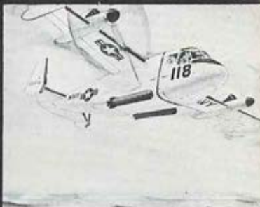
In anti-submarine warfare, the tilt-wing design offers fast forward speed and hovering ability.
