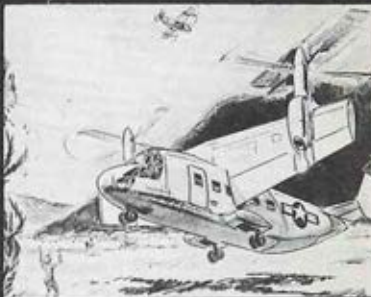
In its dual role as an STOL aircraft, the tilt-wing design could be utilized as a high load capacity air-truck.
