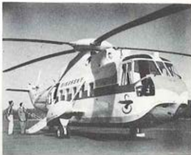
Recently rolled out at the Stratford, Conn., plant of Sikorsky Aircraft, the full-scale static display of the all-weather Sikorsky S-61 is scheduled for initial flight in early 1960. Powered by three turbines, the 56-foot long S-61 features speed in excess of 150 mph, retractable gear, and flying boat hull. The display will be shown at the International Air Salon in Paris from June 12-21.
