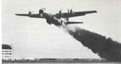
Assisted by 8 JATO bottles, Lockheed's new C-130B Hercules — grossing 135,000 pounds — its maximum takeoff weight and almost 68 tons—roars off Eglin AFB, Fla. runways 2,300 feet from the point of engine run-up. The 350-mile-per-hour troop-and-cargo carrier participated in jet-assisted takeoffs during recent prop-stress tests.
