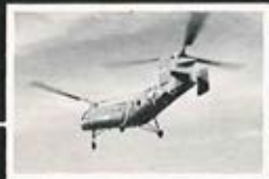
The H-21D research aircraft equipped with two GE T-58 turbo-shaft engines, flown in 1957.
