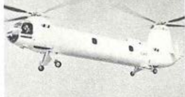
Bristol Type 192 helicopter, which made its first flight on July 5th, is now in production as a troop/cargo carrier and for ambulance and search and rescue duties. The 192 is powered by two 1,300 SHP Napier Gazelle turbine engines, has a cruising speed of 138 mph, and a maximum payload of 6,000 lbs. (Photo/story: SHELL AVIATION NEWS).
