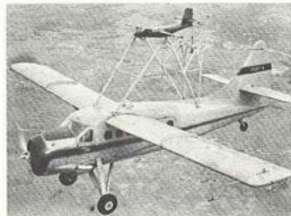
A model of the DHC-4 Caribou, de Havilland of Canada's twin engine utility aircraft, is shown undergoing tests in flight atop a de Havilland Otter flying test bed. Free flight tests of this kind are regarded by de Havilland as a valuable advance on wind tunnel tests. (Shell Aviation News).
