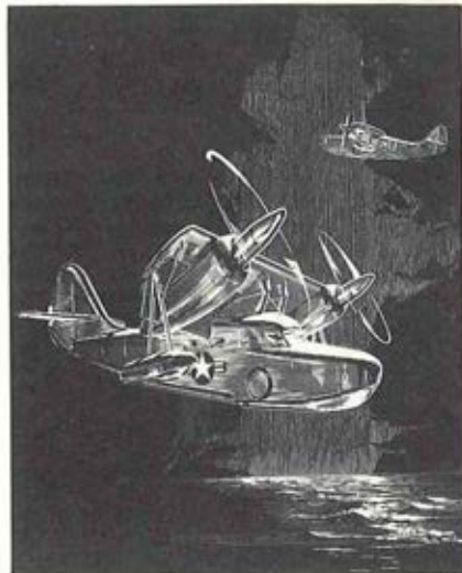
Artist's version of the Kaman K-16B, a VTOL/STOL (combination vertical take-off and landing and short take-off and landing) research aircraft, utilizing the "propeller-rotor" concept being developed by Kaman Aircraft for the United States Navy.
