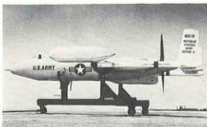
Details of the SD-3 combat surveillance drone being built for the U.S. Army Signal Corps by Republic Aviation Corporation are revealed in this photo of the first model. Developed by the firm's Guided Missile Division, the propeller-driven vehicle uses sensory techniques to keep watch on enemy installations and movements. Capable of zero-length launching, the SD-3 is recoverable. (U.S. Army photo.)
