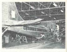
WICHITA, KAN.—Cessna Aircraft Company's 3,000th Model L-19 Bird Dog liaison and observation aircraft has been produced since the airplane first went into production in 1950. Shown moving along Cessna's assembly line in the company's Pawnee Plant in Wichita, Number 3300 is destined for foreign delivery, being one of 53 airplanes ordered by the U.S. Army for the Mutual Dzfense Assistance Program.
