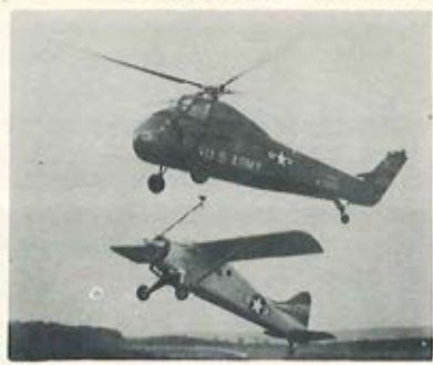
NO JOKE, SONI—An 11th Trans Company Choctaw (H-34 to you) sling-loads a disabled Air Force Beaver to bring the carrier-carried ratio quite close. Spoilers were added to the Beaver's wing to aid the airlift. CWO Henry R. Beau claims a "first" for the 11th in the story below (US Army photo).
