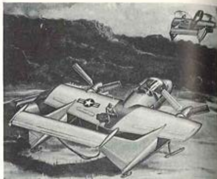
ARTIST'S VERSION of a STOVL aircraft utilizing the propulsive rotor concept being developed by Kaman Aircraft for the U.S. Navy. Small controllable flaps, visible on the trailing edges of the propulsive rotor blades, would provide pilot-control through the 0-50 mph range following which conventional controls would take over. Large Fowler flaps would provide additional lift. The Kaman STOVL would employ gas turbines to power the propulsive rotors and would have a 0-300 mph range (Kaman photo).
